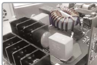
Built-in EMC filter (C2 Class)
